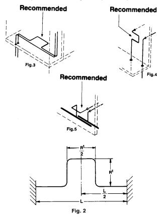
An expansion loop (which is fabricated with 90° elbows and straight pipe as depicted in Fig. 2) is simply a double offset designed into an otherwise straight run of pipe. The length for each of the two loop legs (R'), required to accommodate the expected expansion and contraction in the pipe run (L), may be determined by modification of the SINGLE OFFSET FORMULA to produce a LOOP FORMULA, as shown below:
