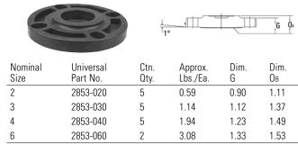
Note: One-piece webbed flanges have oblong bolt holes which permit mating with ANSI B16.5, 150 lb.; BS 1560, class 150; ISO 2084, PN10; and DIN 2532, PN10.
